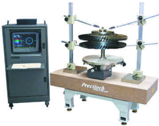
SPS 1000T "high boy" primarily for piece part inspection.
