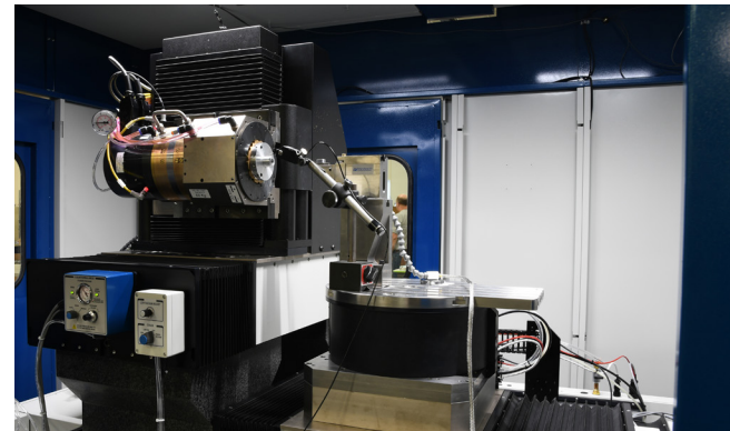
Work envelope. Granite risers used to elevate the X axis, minimizing ABBE offset errors
