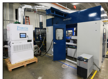
Available with Praecis air shower for up to ±0.01°C temperature control accuracy
