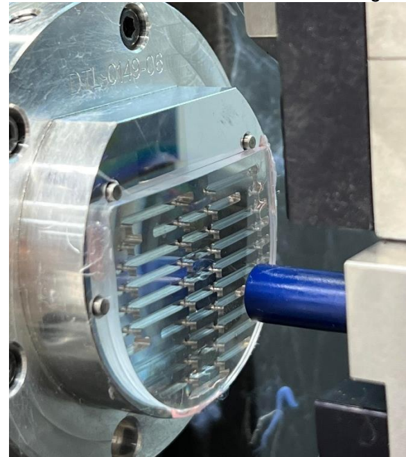
FIGURE 3. Photograph of aspheric PMMA lens on vacuum chuck with asymmetric aperture. The measurement probe is the blue cylinder to the right.
