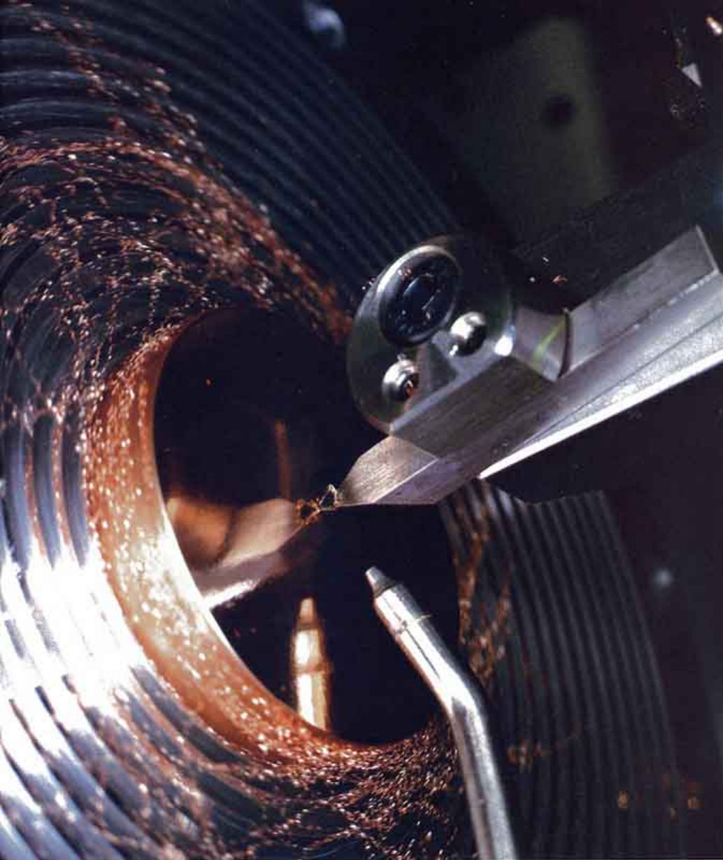
Precitech's diamond-tipped tool removes slivers of copper, creating an industrial mirror.
